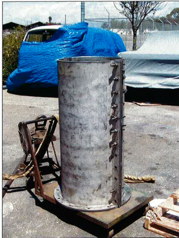
Photo 4 - End sleeve prior to installation.
