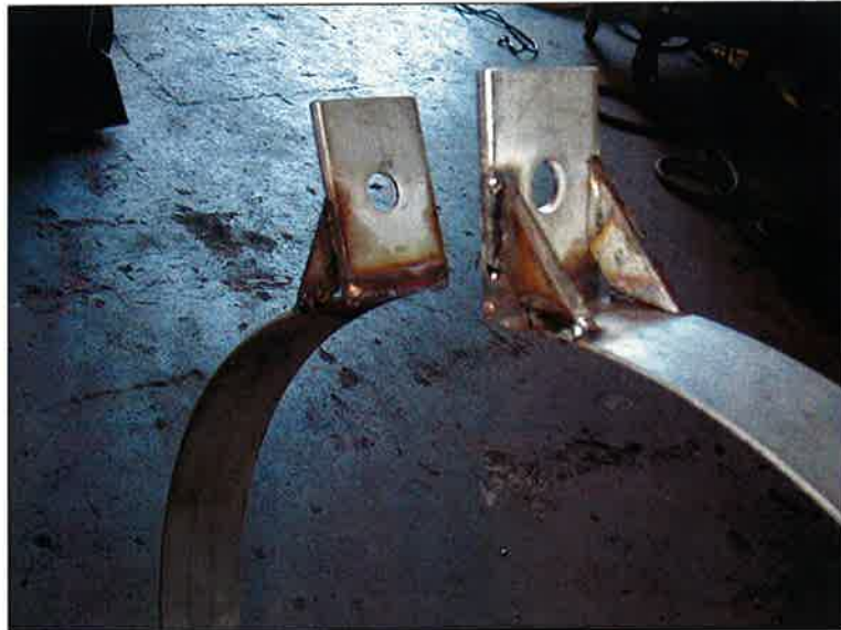
Photo 2 - SS Bands used to secure diffuser saddles
