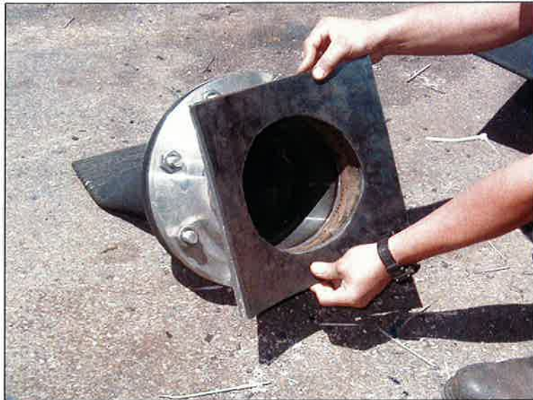
Photo 1 - Gasket glued to sealing face of the valve saddle.
