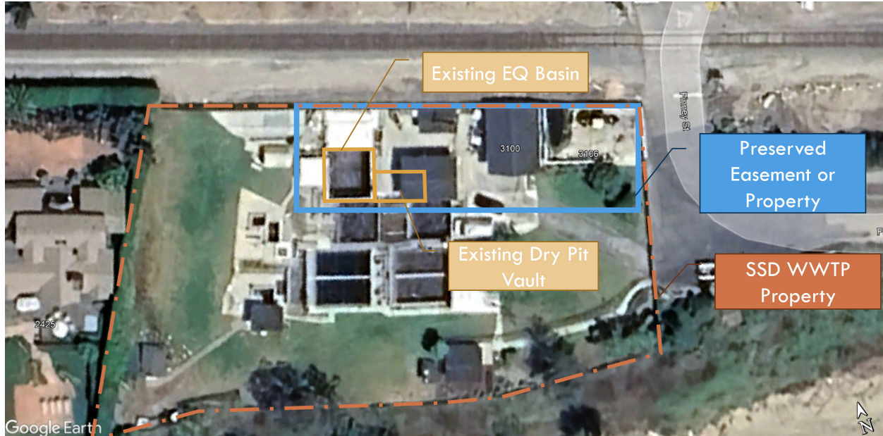
Figure 16 SSD Pumping Facility Conceptual Layout
