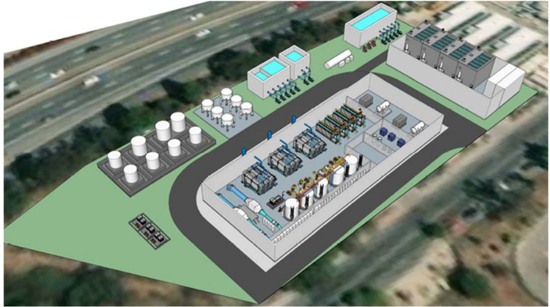
Figure ES.14 Potential Layout for New Advanced Water Purification Facility in Santa Barbara
