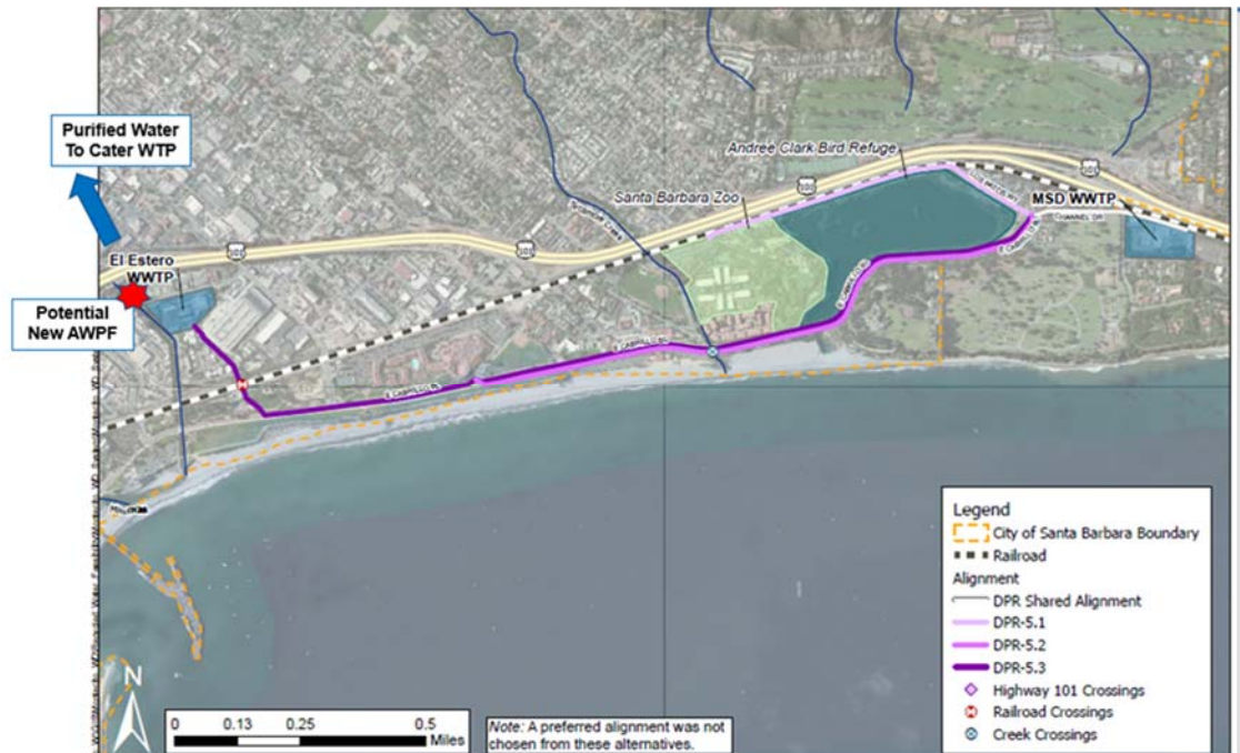
Figure ES.15 Potential Alignments for Sending Raw Wastewater or Secondary Effluent to Santa Barbara's Wastewater Treatment Plant
