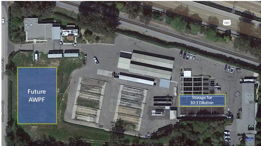
Figure 8.7 Overall Site Plan for DPR at MSD. Site plan assumes the use of retrofit MBR for Treatment Train 4A.
