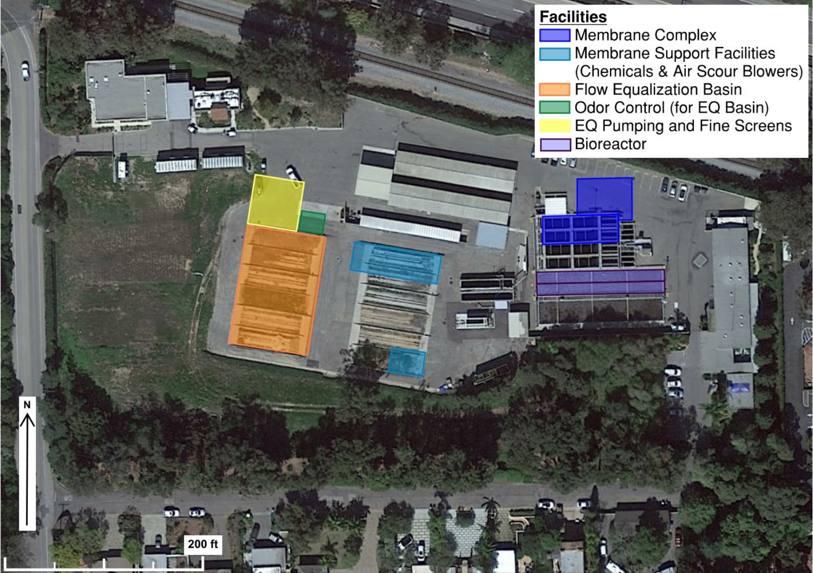
Figure 6.3 Alternative 2 Retrofit WWTP Site Layout
